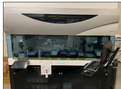
The Tecan robot automatically extracts viral RNA from samples. Startup has been delayed by lack of plastics notably the deep-well plates.
